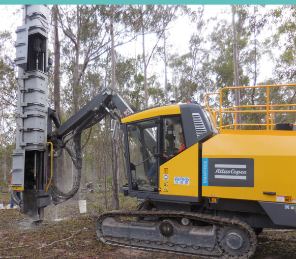
A percussion drill being used to sample the hard-rock resource to a depth of 25 metres; DAF staff provided assistance through site set-up, logistics and supporting field sampling activities
